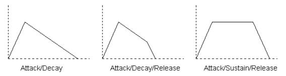
Attack/Decay - this is useful for percussive sounds such as plucked strings, drumbeats etc. Set the *Sustain Volume* and *Release Time* to zero. Make sure that the sum of the Attack and Delay times is equal to the sound duration (set by the <u>Output component</u>).
