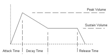
The envelope generated will always occupy the full duration of the file. The times of the Attack, Decay and Release phases are fixed, but the Sustain time is not. The Sustain time will be automatically adjusted so that the total time of all 4 phases is equal to the duration of the sound.
