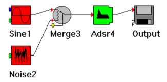
Notice that several inputs are not connected. For example, the Sinewave Generator *Frequency* input is not connected. This simply means that the frequency is not controlled by an external source, it remains constant at 1000 (the value we set when we created the component).
