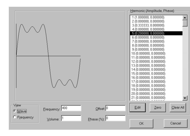
The overall *Phase* may be altered so that the wave begins at a different point in its cycle. This takes a value of 0% to 100%, which advances the wave in time by a fraction of a complete cycle.
