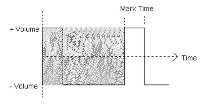
The signal oscillates between two extreme values (given by plus *Volume* and minus *Volume*). Initially, the wave starts at the high value, as shown in the diagram. The shaded area represents one complete wave period.
