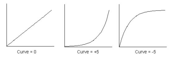
In the first case, with a curve of zero, th rise (or fall) of volume is linear with time.
