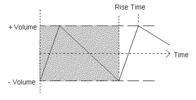
The signal oscillates between two extreme values (given by plus *Volume* and minus *Volume*). Initially, the wave starts at the lowest value, as shown in the diagram. The shaded area represents one complete wave period.
