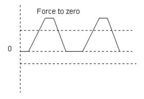
Symmetrical clipping applies an equivalent clip to both positive and negative going signals. Clip levels must be positive for symmetrical clips. In the diagram below, the lower level cliping is used in conjunction with *Force to zero*.
