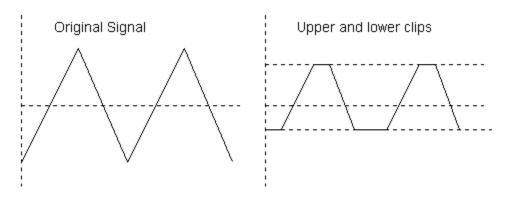
*Force to zero* has the effect of shifting the signal so that the lower level clipped signal is at zero level (mathematically, it subtracts the Lower Level Cutoff value from the clipped signal).
