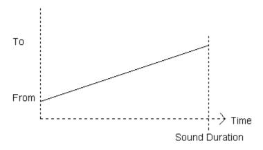
The signal may increase (as shown) or decrease with time, depending on whether the *To* value is greter than or less than the *From* value.
